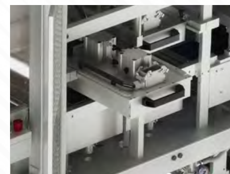
Tool-free die changing in less than 2 minutes.
