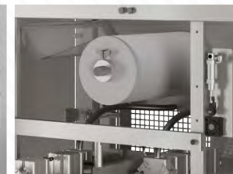
Automatic film rewinder with motor-driven film reel shaft and film waste shaft. Inverter-controlled shaft acceleration and deceleration times.
