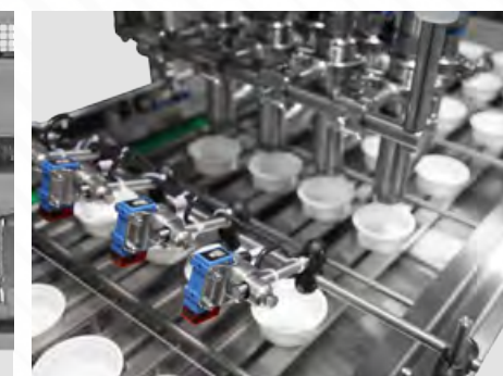
Automatic dosing of solids, liquids and granules.
