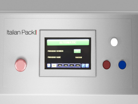
Plc Omron Touch wide screen 7.2" a colori, porte USB/ethernet, 99 programmi, personalizzazione della lingua, controllo temperatura integrato, gestione avanzata parametri MAP, Tray SKIN e graduate vacuum. 7.2" Omron PLC Touch screen, color display, USB port/Ethernet, 99 packaging programs, language selection, integrated temperature control, menu-driven M.A.P. parameters, skin tray and gradual vacuum.
